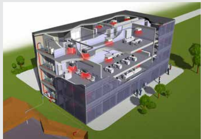
1 Cooling Tower or Dry Cooler 2 Boiler 3 Indoor Units 4 Refrigerant Pipes 5 Condensing Units 6 Water Loop Piping
